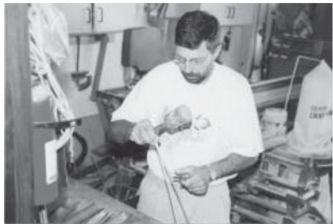
The culm is being split into strips about 1/4 inch wide in preparation for planing.
