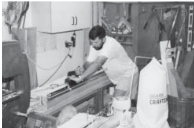
Each strip is planed into a tapered triangular strip about four feet long, depending on rod length. A set of six matching strips is glued together to form the hexagonal rod section.
