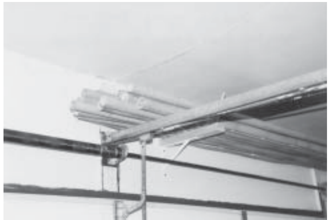
Culms that are in the process of aging. These are imported from China and each will make one or two rods. They are twelve feet long and about 2 1/2 inches in diameter. They age two to five years before Bill uses them.
