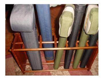
To keep the rod cases from moving from side to side I created dividers out of strips of wood which wrap around the dowel rods and are secured by a bolt on each side. I used wing nuts so the distance between dividers is easily adjustable. These strips were created by centering a hole in the middle of a strip of wood and a hole at each end for the bolts before ripping it in half so as to be able to place them around the doll rod.
