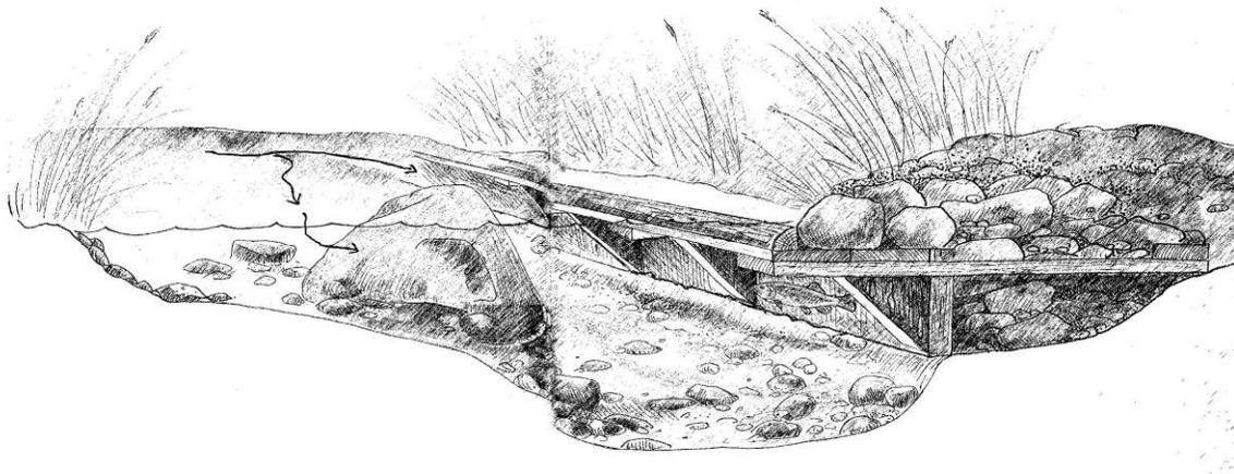
A drawing of an installed skyhook
