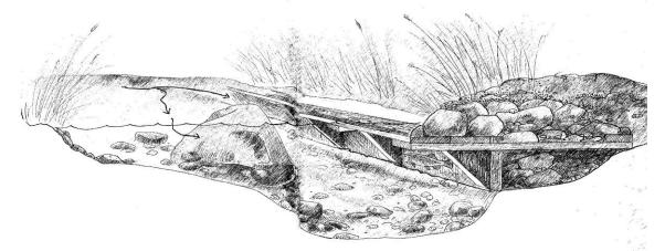
Skyhooks will be the main structures installed on the Bohigian CA portion of Mill Creek. Skyhooks are structures designed to increase the amount of overhead bank cover for trout. They are assembled out of rough cut green oak on the stream site and then set into the bank. Large rock is then installed to armor the structures and stabilize the bank.
